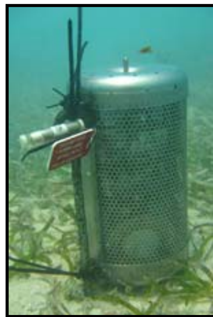
Figure 3.6. POCIS and SPMD sampler attached to a stake. An acoustic transmitter was attached to the sampler to allow retrieval in turbid conditions.
