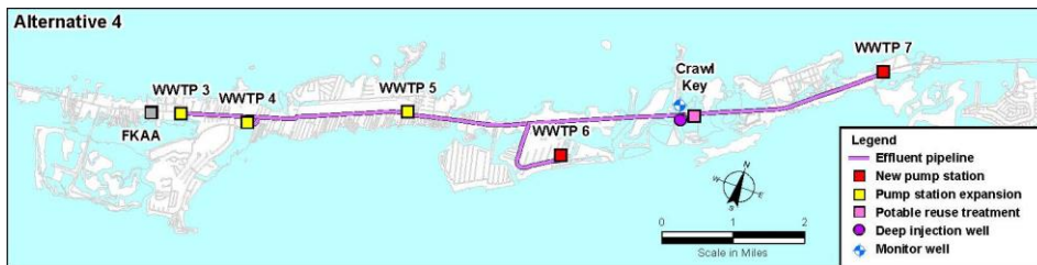
Figure 3.10: Alternative 4 Direct Potable Reuse
