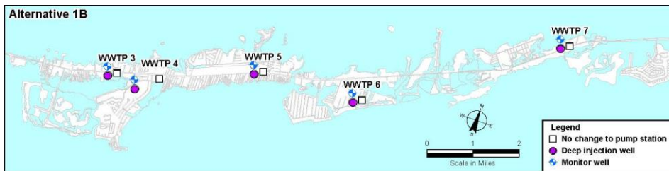
Figure 3.4 – Alternative 1B Five Deep Injection Wells
