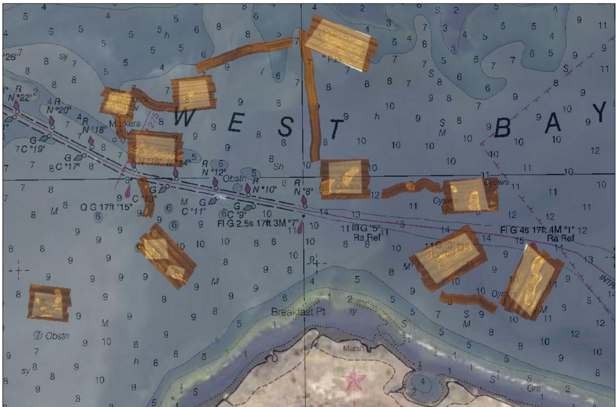
Figure 7. A view of the western parts of West Bay provides a representative example of how the initial acoustic imagery coverage was focused on obtaining at least 100% imagery coverage over all of the defined “oyster” polygons. In this figure, the imagery mosaics are partially transparent so the underlying polygons are visible. Additional acoustic data were also acquired during transits between the primary areas.
