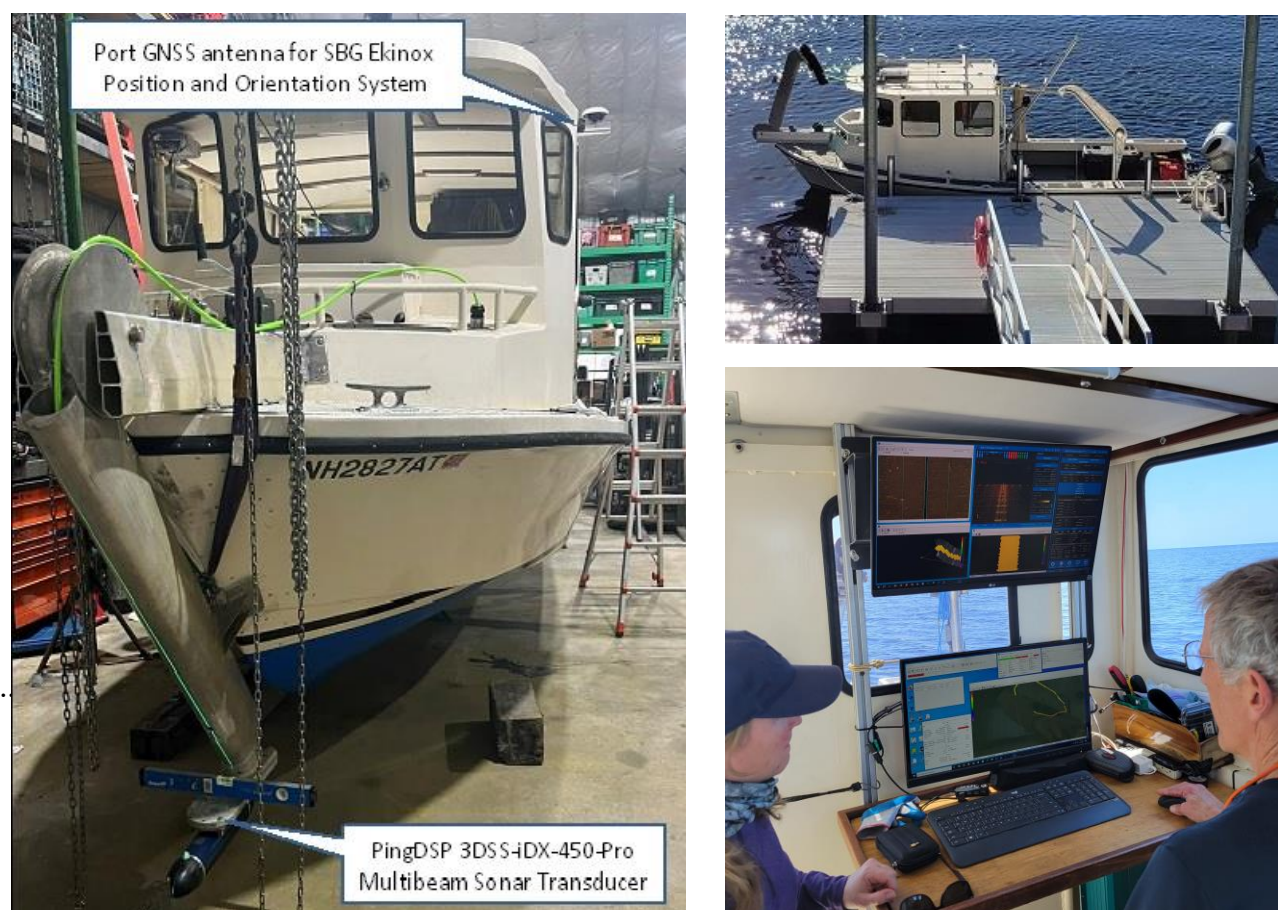
Figure 3. Left: Acoustic gear on Substructure's Diversity with bow-mount and towfish in deployment position. Top: Diversity dockside with bow-mount in raised position for transport. Lower: Sonar monitors in Wheelhouse.
