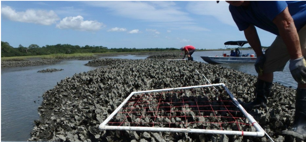
Figure 2. A point-intercept quadrat for measuring percent cover on an intertidal oyster reef. Credit: GTMNERR.
