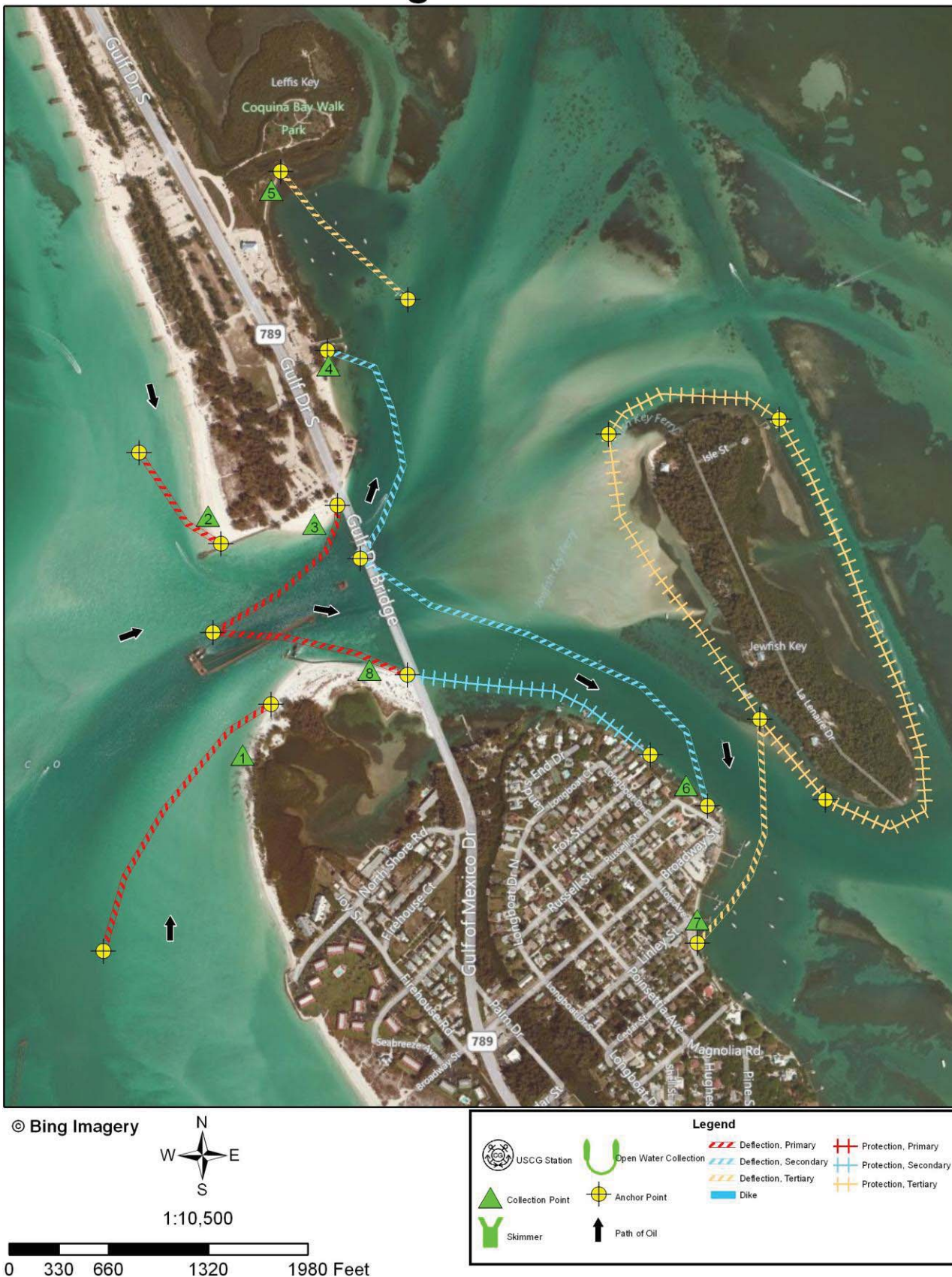
FIGURE 6. Flood-tide protection strategy recommended for Longboat Pass.
