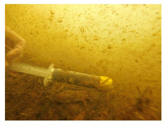
Figure 4.2: Unstable, low-density sediments of impaired canals can easily be disturbed. Note the dead leaves and plant detritus that dominate surface sediments rather than expected sand grains. The pictured device was used to remove cores of surface sediment for laboratory analysis.
