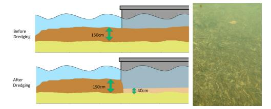
Figure 3.35: Left - Diagram depicting excess of wrack remaining outside Canal 266 after interior was dredged. Right - Photo of seagrass wrack accumulated outside canal mouth.
