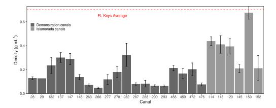
Figure 3.6: Values of sediment density (measured as dry bulk density) during the first year of monitoring, prior to demonstration technologies. Values represent mean ± SE compared to the average (red line) for natural waters in the FL Keys from Howard, 2018.
