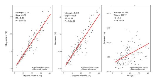
Figure 3.8: Correlations between percent organic material and C<sub>org</sub>, N, and P content of sediments. There is a significant, positive relationship between all of the presented variables.
