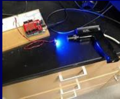
Benchtop fluorometer prototype testing of LED emitter with light spectra output to computer
